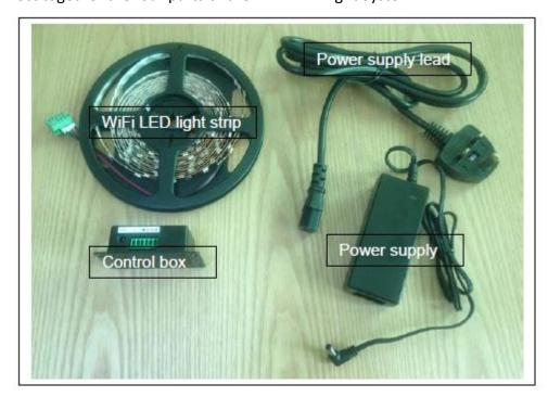
3. Plug the end of the Wi Fi LED light strip into the black control box:
