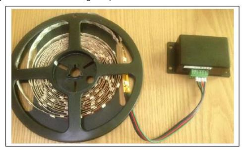
4. Plug the power supply jack into the black control box:
