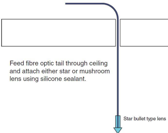
Feed fibre optic tail through ceiling and attach either star or mushroom lens using silicone sealant.
