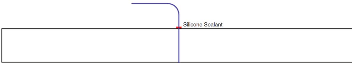
Feed fibre tails through the holes in the ceiling, leaving approx. 150mm in length protruding. This will allow for painting prior to the tails being trimmed.
